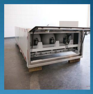
3 cylinder skid capable of transporting ~300 SCM of product / Working pressure is 43.1mPa (431 BAR) (6250 PSIG) Skids weigh under 2100 Lbs
